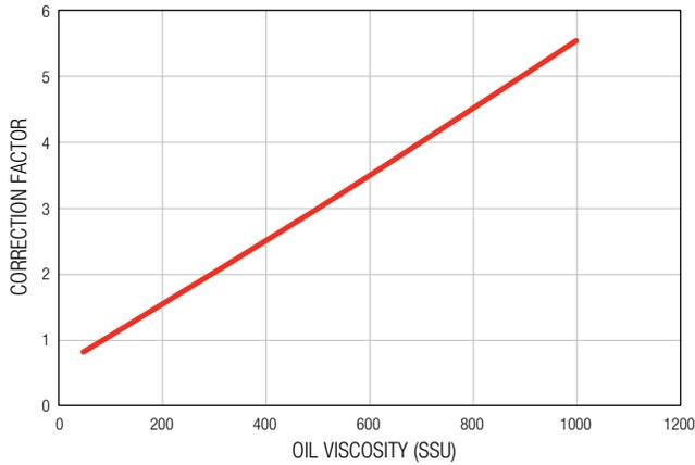
Performance Curves are based on 100SSU oil at 40°F approach temperature (125°F oil leaving cooler, 85°F water entering cooler), 2:1 oil: water ratio (1 GPM water flow for each 2 GPM oil flow).
