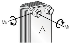
The maximum allowable connection loads given below are valid for low cycle fatigue. If high cycle fatigue is involved special analysis should be made.
