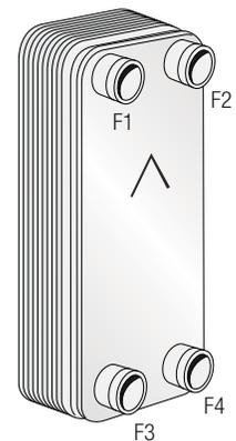
Ports F1/F2/F3/F4 are situated on the front of the heat exchanger.
