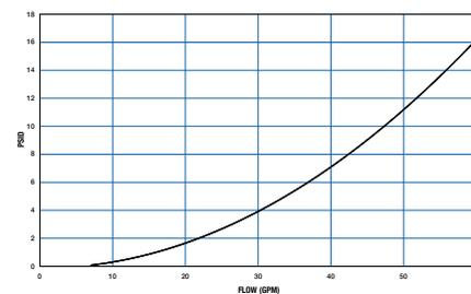
Inlet Port Over Integral Relief Valve @ 170°F (78 SUS)
