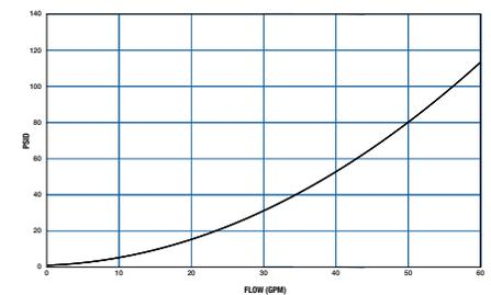
NOTE: Pressure drop shown is added to relief valve crack pressure for total pressure drop.
