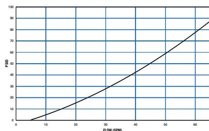
Inlet Port Thru Cooler Port @ 145°F (110 SUS)
