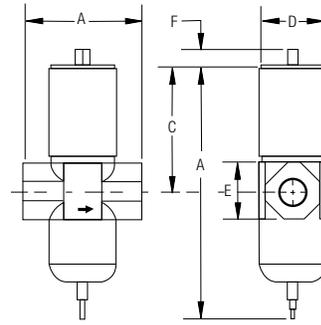
Standard temperature elements are furnished with 6' capillary. Longer capillary lengths not available. Valve Disc: Buna N in brass disc retainer.
