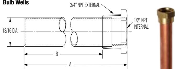
65187 Half Coupling - Mount to Reservoir. For use with all bulb wells shown above.
